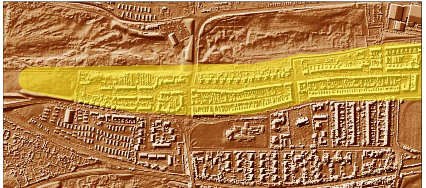
Lidar scan showing the topography of Coatham with the location of the sandbank described in 2.2 highlighted in yellow
