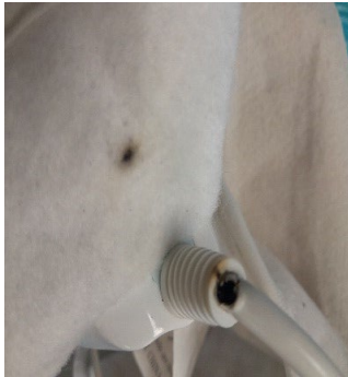
Electric blanket that failed testing
