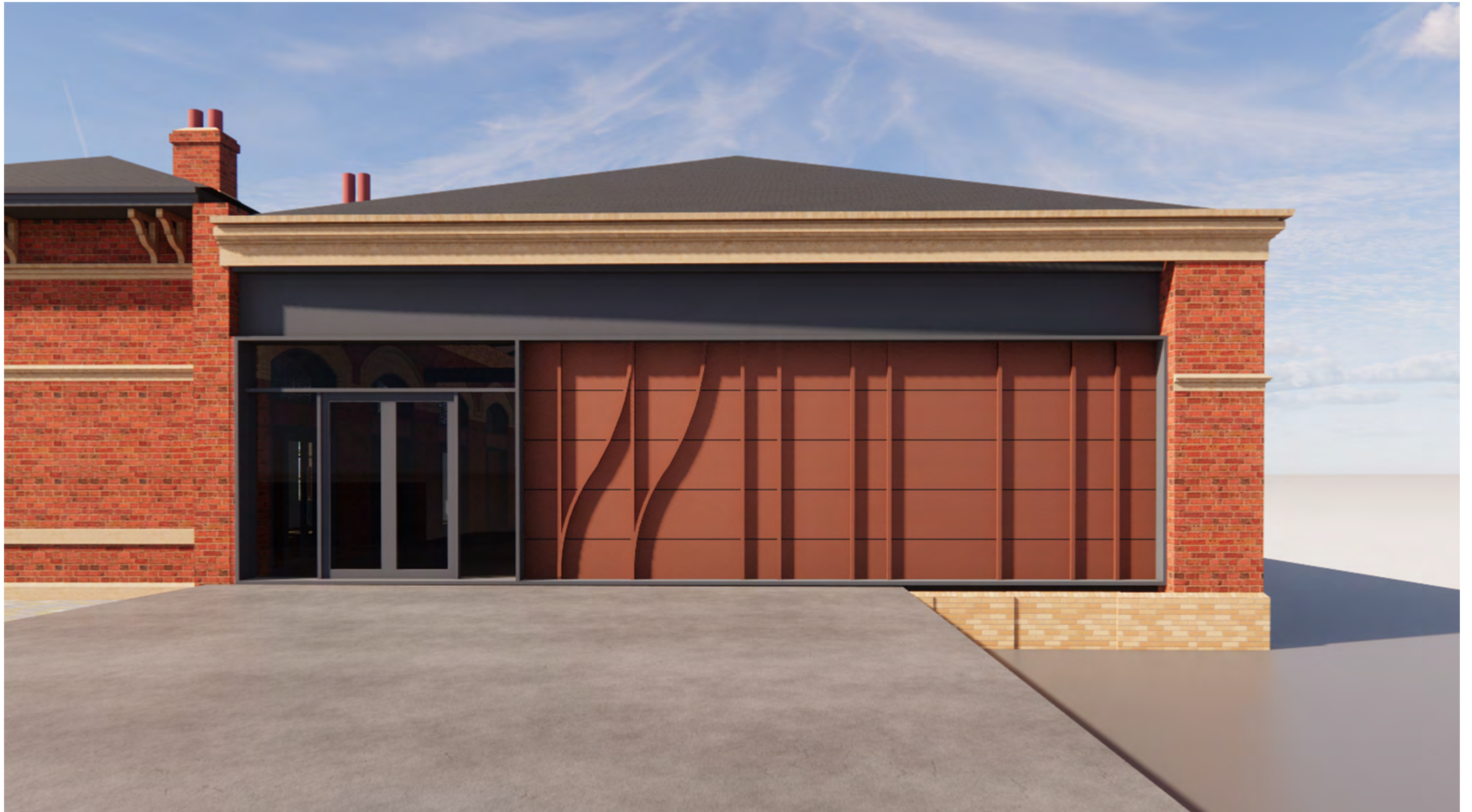
Figure 59. Train Shed Redesign Option B - Curtain walling structure with COR-TEN panels and transoms resembling rail tracks. The width between the transoms corresponds to the standard gauge distance
