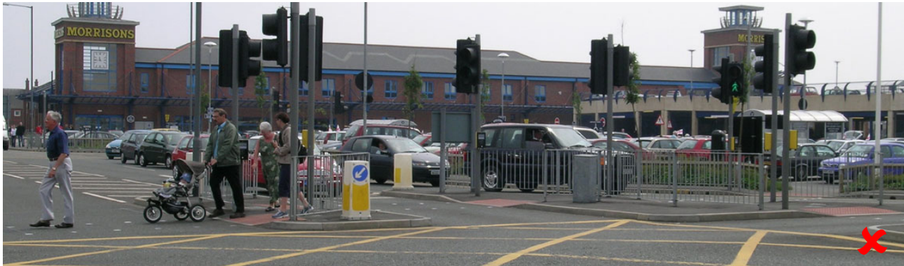
Fig 132. A road layout conceived primarily with motorists in mind has resulted in a pedestrian-hostile environment and a sea of traffic lights, barriers and infrastructure.
