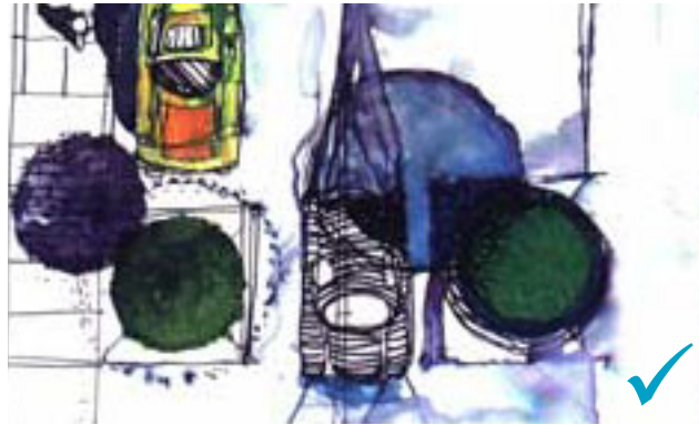
Fig 104. Trees can be planted as part of a traffic calming or street enhancement scheme. Here they are planted in the 'nib' designed to slow traffic entering a residential area..
