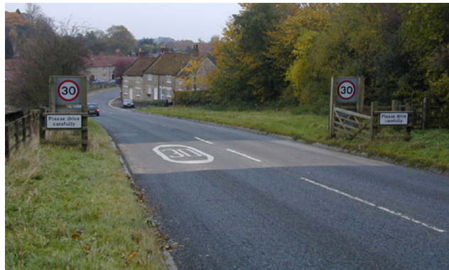
Fig.147. A reasonable attempt at rural Helmsley to achieve a similar effect at a new 'village gateway'
