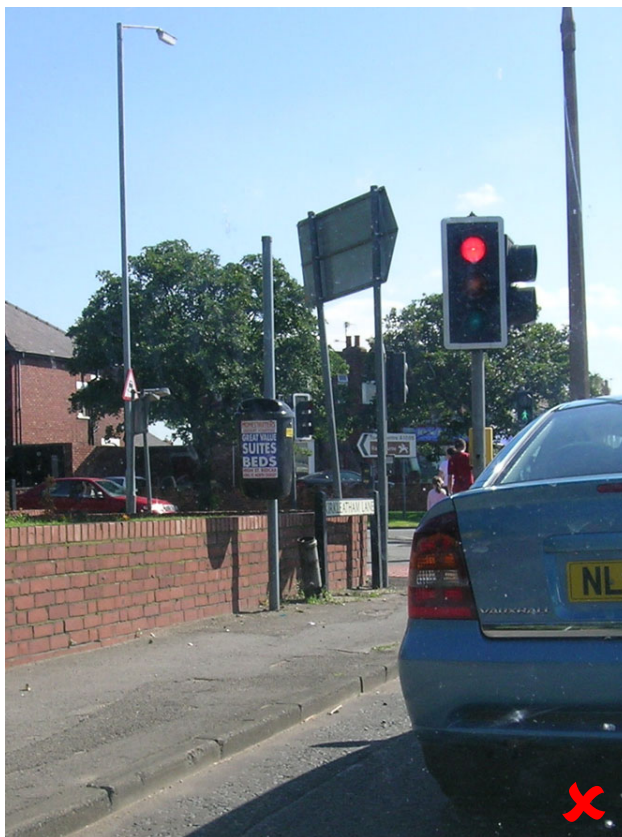
Fig 117. A clutter of poles; a broken light column stub; pole mounted nameplate; and, bent signage. The gateway to Redcar at Locke Park. Such examples can be found throughout the Borough and hinder attempts to achieve a quality environment.
